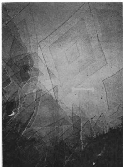
Figure 17 —Further consequences of heating the crystals in Figure 15 in suspension at 0.3 deg. C/min to between 89°C and 92°C; dissolved polymer has recrystallized on cooling to give regular lamellae once more
