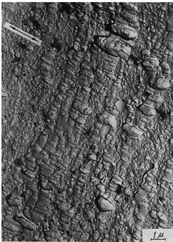
Figure 3 —Electron micrograph of whitening induced by a tensile stress applied to the specimen shown in Figure 2 . Crazing associated with deformation of rubber particles is demonstrated. Arrow indicates direction of the applied stress
