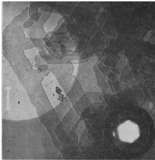
Figure 11—Selected area diffraction pattern of crystals from n -dodecane (1 000 minutes at 95°C, then 1 000 minutes annealing at 105°C)
