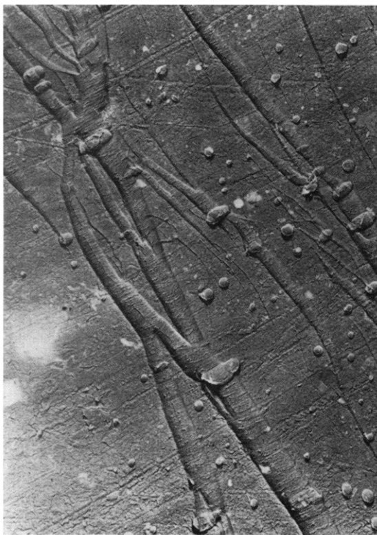
Figure 1 —Electron micrograph of stress-whitened surface of compression-moulded sheet of HI-PS showing branched crazes. Direction of applied stress is perpendicular to main craze axis. Scale as Figure 3
